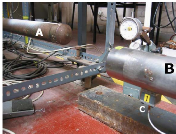
Fig. 2. Impact rod (A), long pipe (B) and pressure transducer “pt1” (C).
